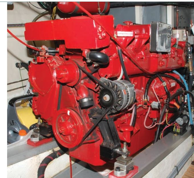
Well maintained, properly sized for the application, and operated within the optimal minimum and maximum loads, this engine has a good shot at running for 10,000 hours—and possibly much more.
